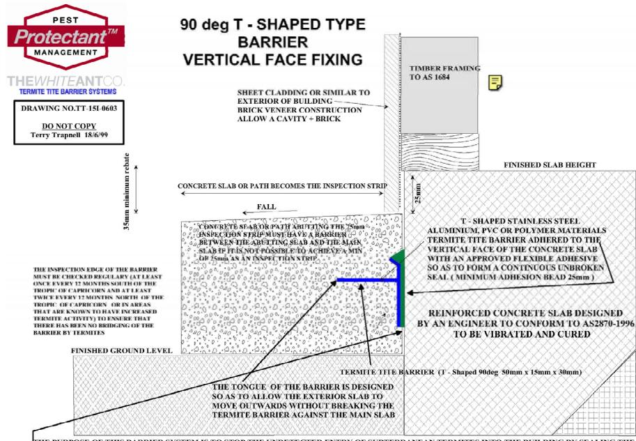
THE PURPOSE OF THIS BARRIER SYSTEM IS TO STOP THE UNDETECTED ENTRY OF SUBTERRANEAN TERMITES INTO THE BUILDING BY SEALING THE COLD JOINT BETWEEN THE EXTERIOR CONCRETE SLAB / PATH AND THE BUILDING SLAB - THE EXTERIOR SLAB THEN BECOMES THE VISIBLE INSPECTION AREA ALLOWING THE DETECTION OF ANY TERMITE ACTIVITY - MININIUM ABUTTING SLAB WIDTH AND DEPTH IS 100mm.
