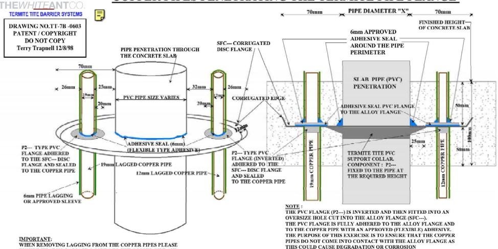
WHEN REMOVING LAGGING FROM THE COPPER PIPES PLEASE ENSURE THAT NO DAMAGE OCCURS TO THE COPPER PIPE AND THAT THE LAGGING IS REPLACED TO ITS ORIGINAL CONDITION OR THE PIPE SLEEVED TO ENSURE THAT NO CONCRETE COMES IN CONTACT WITH THE COPPER AS THIS WILL CAUSE THE COPPER PIPE TO CORRODE
